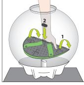
5. Fold the matting and support in half and insert into the tank, opening out with the matting on top (1). Check it's flat against the base then fit the rubber stopper supplied with the matting (2).
