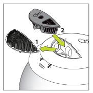
**12.** To install the air filter, remove the air filter cover (1), unwrap and place the air filter in the cavity (2) and replace cover.
