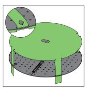
4. Fix the capillary matting to the support tray and secure onto the buttons as shown.Making sure the centre holes line up.
