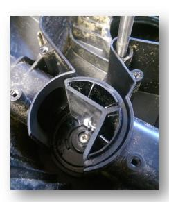
The twist grip is now fitted and should work correctly. Refit the lid assembly using the screws put aside, the foams can then be reattached and the base plate refitted.
