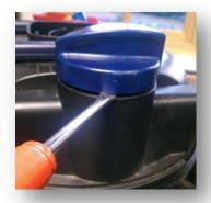
Once the blue handle and the diverter valve are removed, ensure that both of the old o-rings that create the water tight seal are also removed, these can all be disposed of as the new pack will contain these.
