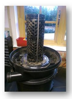
First remove the UVC unit; this can be done by pushing the blue safety clip and turning anti-clockwise. Ensure that the easy clean handle is fully depressed to allow removal of the unit.
