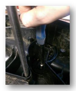
The diverter valve can now be removed, using the Philips screwdriver, take out the screw and pull out the valve.
