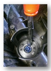
Place the blue handle in position and press over the orings; this can be made easier if a flat head screwdriver and some grease are used.
