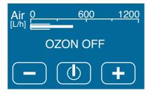
The upper bar graph (»Air«) indicates the amount of airflow through the ozonizer in litres per hour.
