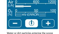
generator may cause damage, creating a faulty voltage potential inside the ozonizer. In this event, please disconnect the ozonizer from the power supply immediately, removing the wall plug from the mains socket. Blowing air through the ozonizer may remove any water that has entered. Please cleanse the ozone generator as described above. If the problem persists, please send the ozonizer in for inspection at Sander company headquarters (see address on back cover page).
