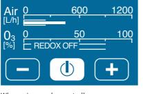
When using a redox controller, ozone production is turned off automatically once the target redox potential set on the redox controller has been reached. When the redox potential drops below the set value, ozone production is resumed.
