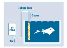
The ozonizer may be installed in an equipment cabinet. If the ozonizer is operated in a small enclosed space such as a cabinet, it is essential to provide sufficient ventilation to avoid overheating. If the ozonizer is installed below the water level, provide a loop of tubing extending above the water level to avoid water flowing back into the ozonizer.
