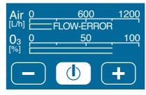
If airflow through the ozonizer drops below 75 litres per hour, ozone production will shut down to prevent overheating. Please provide sufficient airflow to the ozonizer, removing any blockages.
